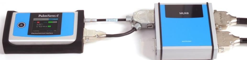
*PalmSens4 connected to MUX8-R2 multiplexer*
