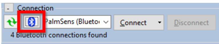
4. All available PalmSens Bluetooth devices will be listed. The last four characters of each device name are the last four characters of the Bluetooth MAC address. This address can be found on the bottom of the extension module.
