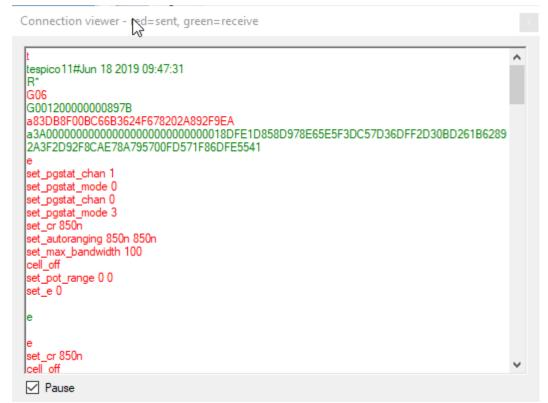
The connection viewer window. All information in red is sent from the PC to the device and the green information is sent by device to the device.
