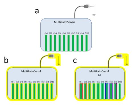
Figure 2.1 a) Scheme of a MultiPalmSens4 with its PCBs; b) MultiPalmSens4 with yellow halo indicating the same ground; c) MultiPalmSens4 with Galvanic Isolation and indication of different ground by different colored halos
