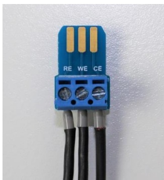
Figure 3.1 Screw terminal with marks for the electrode connections
