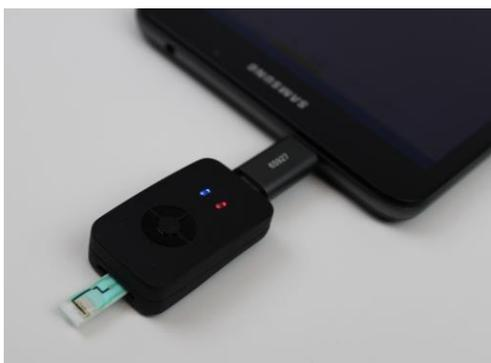
Figure 3.2 Sensit Smart and glucose sensor during the measurement
