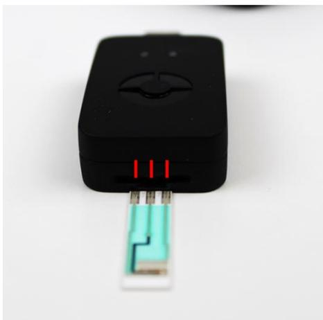
Figure 3.1 Front of the Sensit Smart with highlighted grooves
