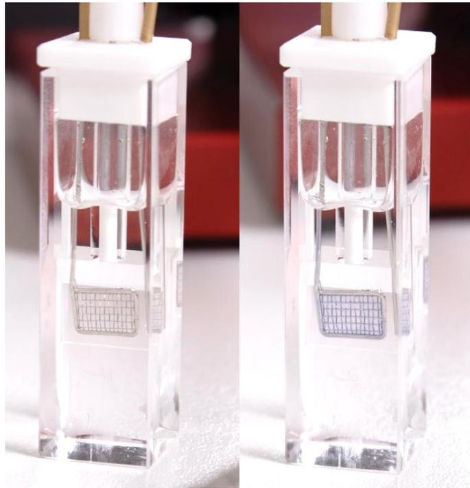
The platinum mesh changes color by applying a voltage.
