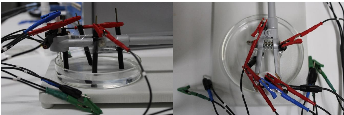
Figure 2 A setup with 4 working electrodes, 1 reference electrode, and 1 counter electrode (left side view, right top view)
