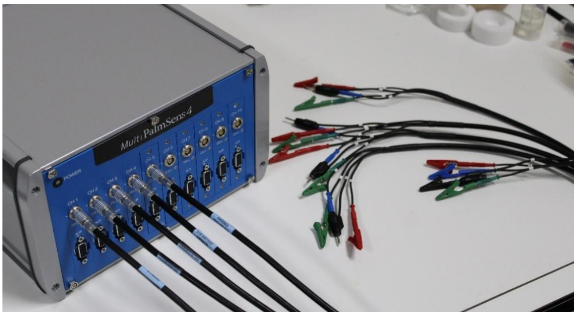
Figure 4 MultiPalmSens4 with reference and counter electrode leads for each channel connected to each other except for channel 1
