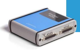
The MUX8-R2 multiplexer is also available with integrated EmStat3 or EmStat4 potentiostat. This very compact combination allows for a high productivity with a small footprint.
