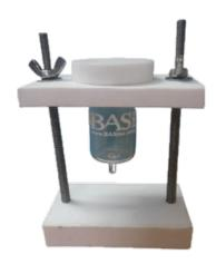
Exposed Diameter of Specimen: 1 mm. An 0-ring provides reproducible exposed area
