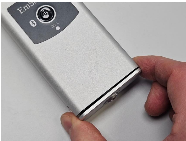
Figure 5 Pulling out the Connection Module.
