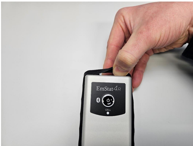
Figure 7 Pulling the rubber sleeve over the back of the housing.
