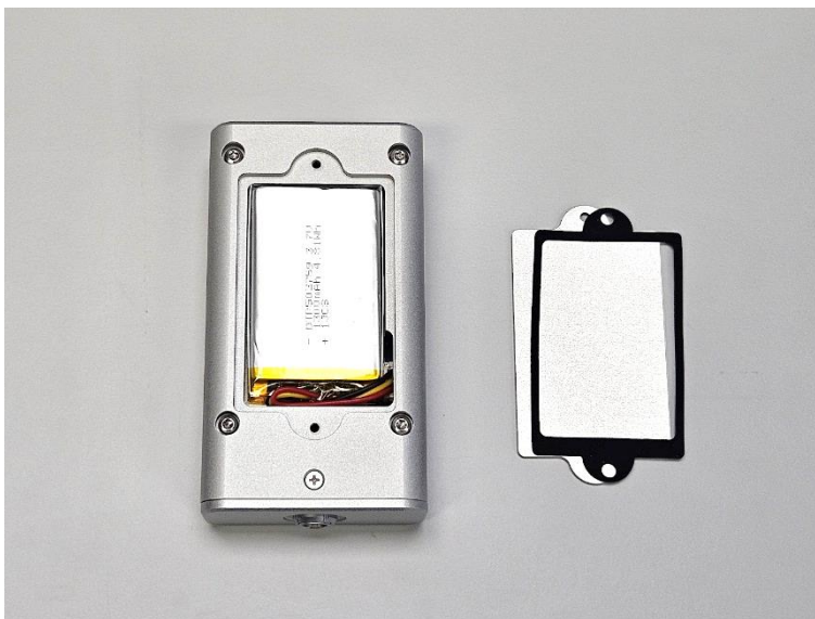
Figure 11 The battery lid removed.
