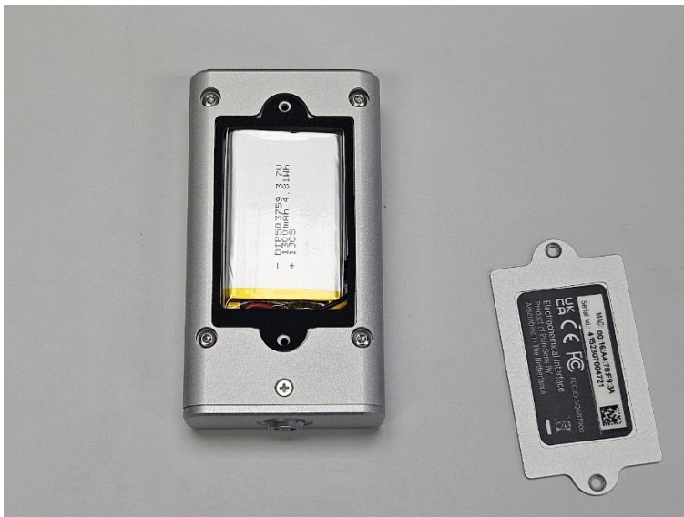
Figure 13 Putting the rubber gasket in place.
