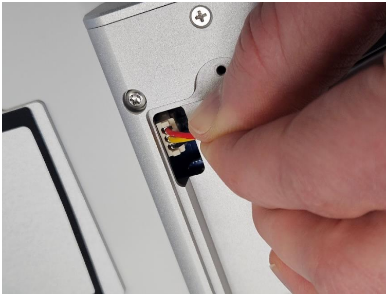
Figure 12 Unplugging the Li-Po battery
