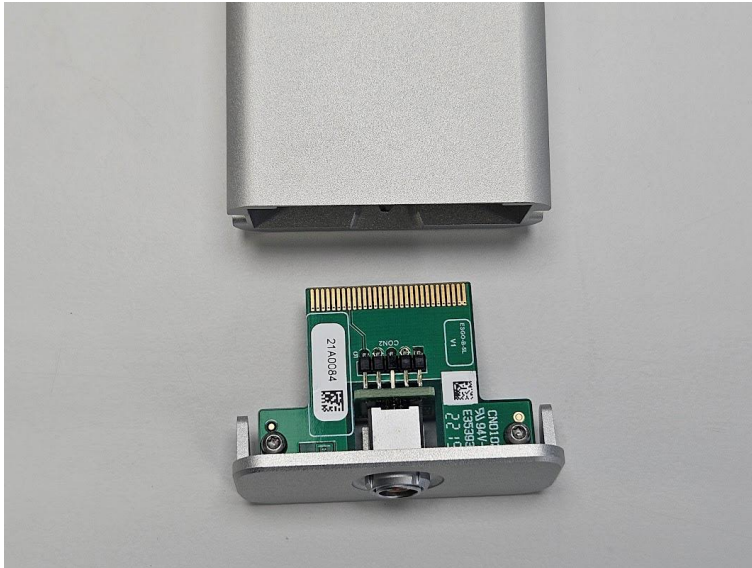
Figure 6 Replacing the Connection Module
