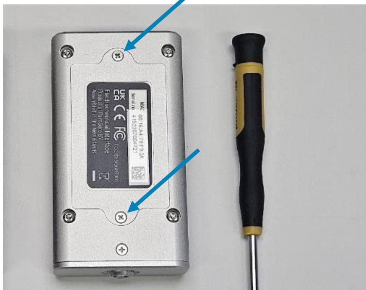
Figure 10 The two screws of the battery lid.
