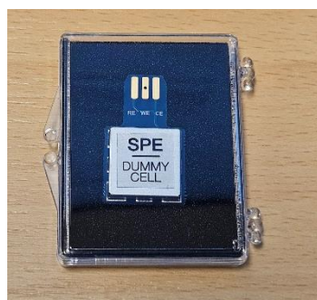
Figure 16 The SPE dummy cell supplied with the EmStat4R SPE version.
