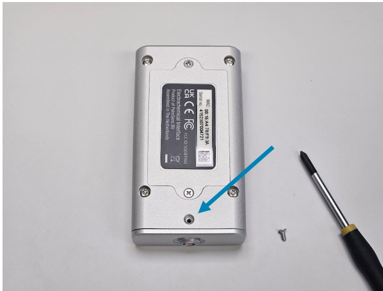
Figure 4 The Connection Module screw location.
