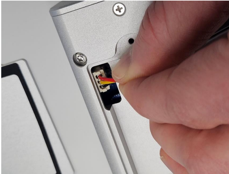
Figure 12 Unplugging the Li-Po battery
