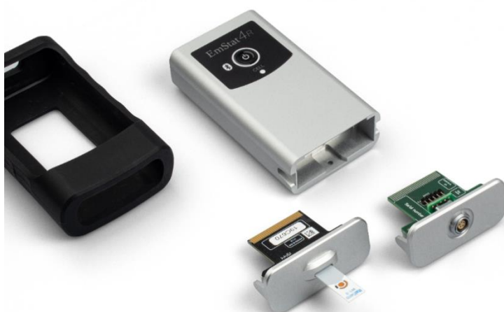
Figure 1 The Connection Module of the EmStat4R can easily be exchanged.
