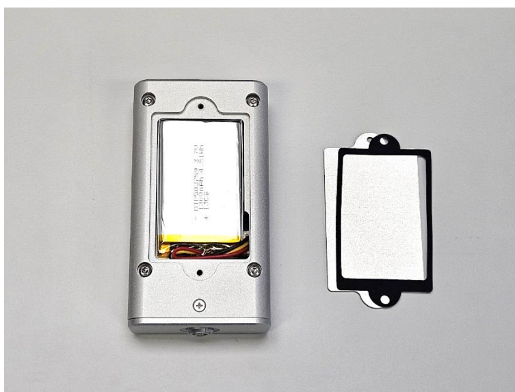
Figure 11 The battery lid removed.
