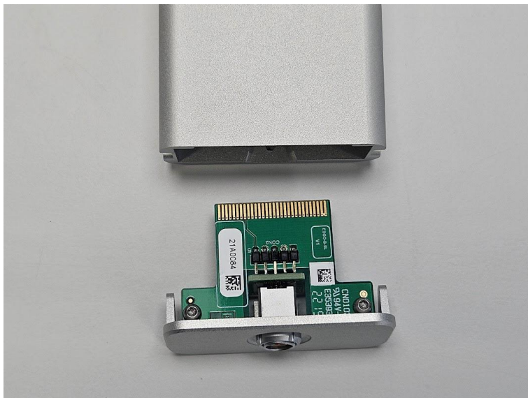
Figure 6 Replacing the Connection Module
