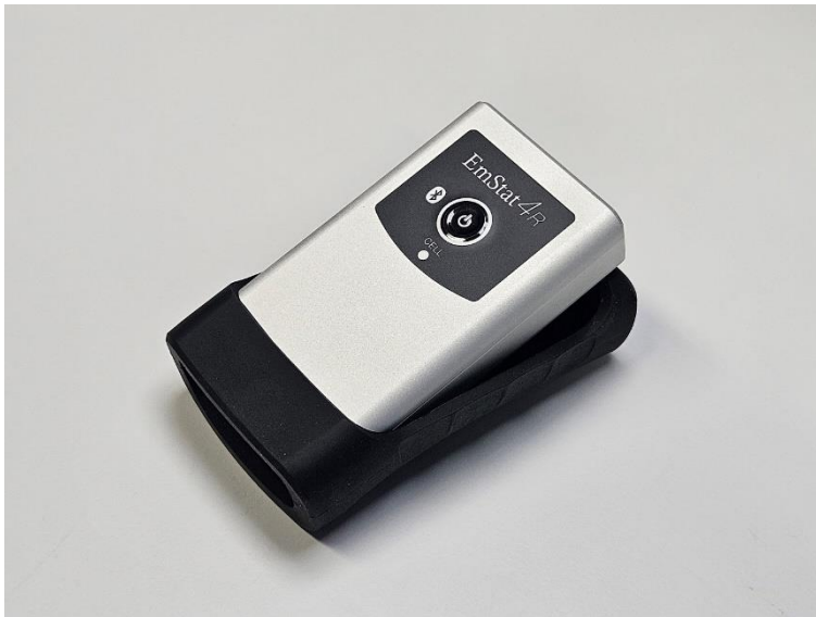
Figure 9 Removing the rubber sleeve.
