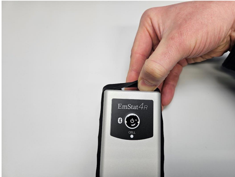
Figure 14 Pulling the rubber sleeve over the back of the housing.
