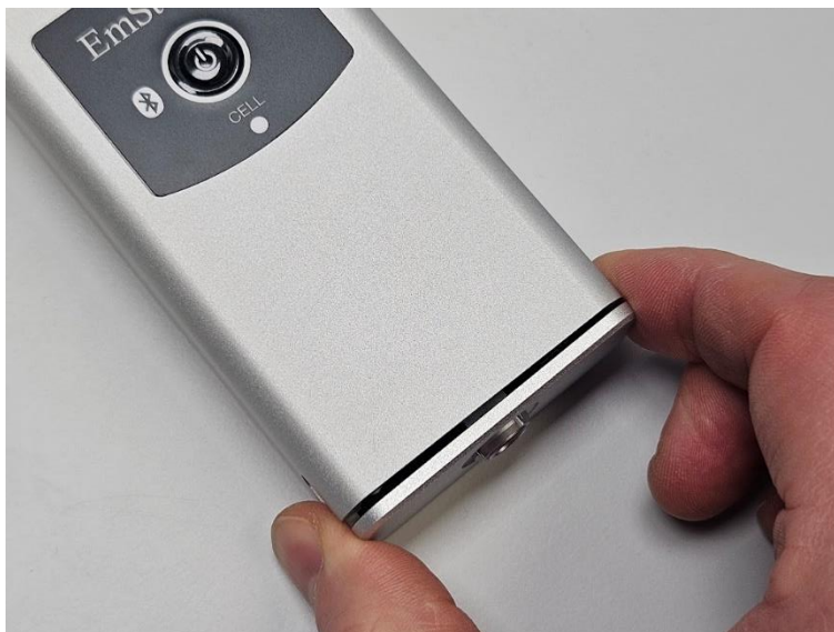
Figure 5 Pulling out the Connection Module.
