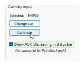
The TMP36 gives a voltage of 10 mV per measured centigrade.
