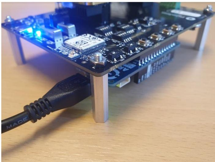
Figure 9 - Powering all stacked boards via the Arduino MKR
