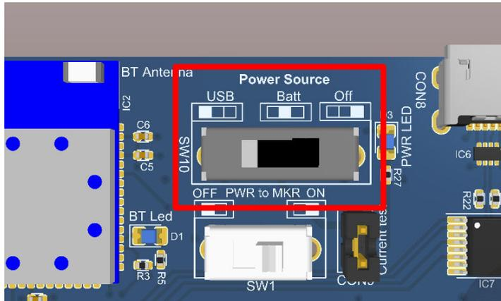
Figure 8 - SW10 on the development board
