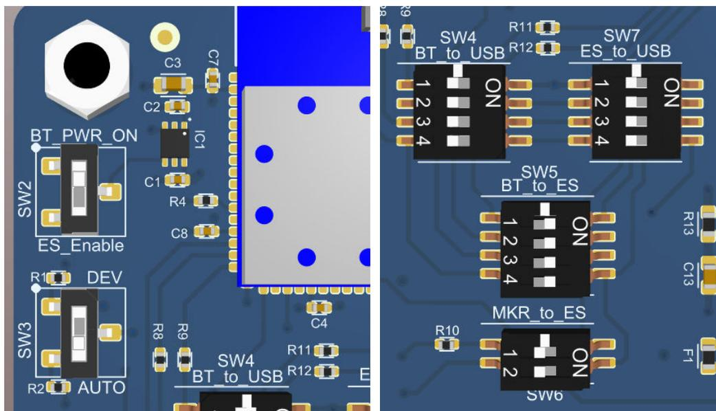
Figure 2 - Dip switch settings for allowing a Bluetooth connection to the EmStat4M module
