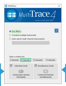
Individual Mode: where each channel can run a measurement or script independently from the other channels.
