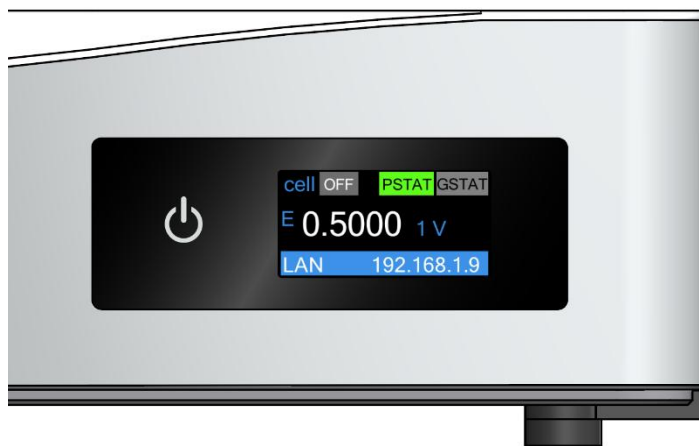
Figure 4 The assigned IP address showing in the blue bar on the display
