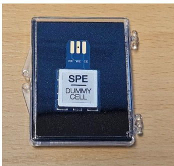
Figure 392 The SPE dummy cell supplied with the EmStat4R SPE version.
