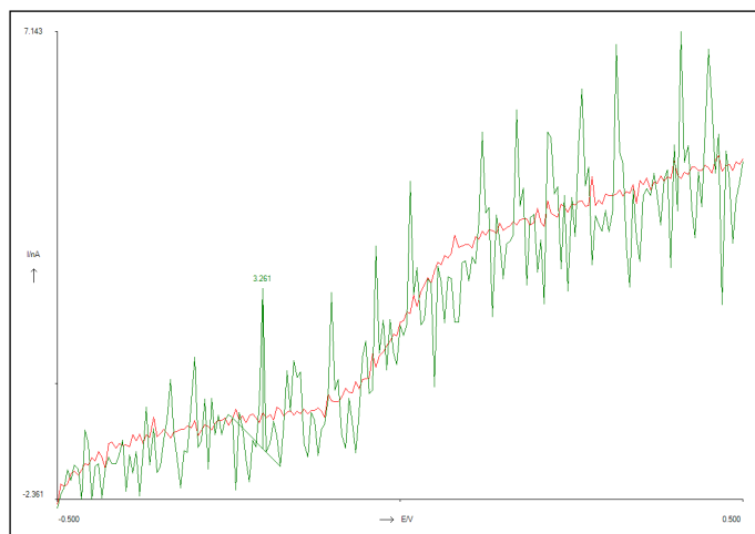
Figure 73 The green (noisy) and red curves are both measured with the same conditions as before and with the same EmStat. The red curve is obtained when EmStat is connected to a USB hub instead of directly to a USB port of the PC.
