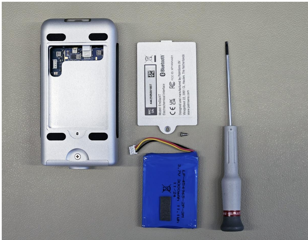
Figure 22 - EmStat4X with the battery lid removed.
