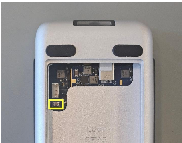
Figure 26 - EmStat4T bootloader emergency button
