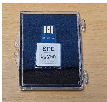
Figure 25 The SPE dummy cell supplied with the EmStat4T SPE
