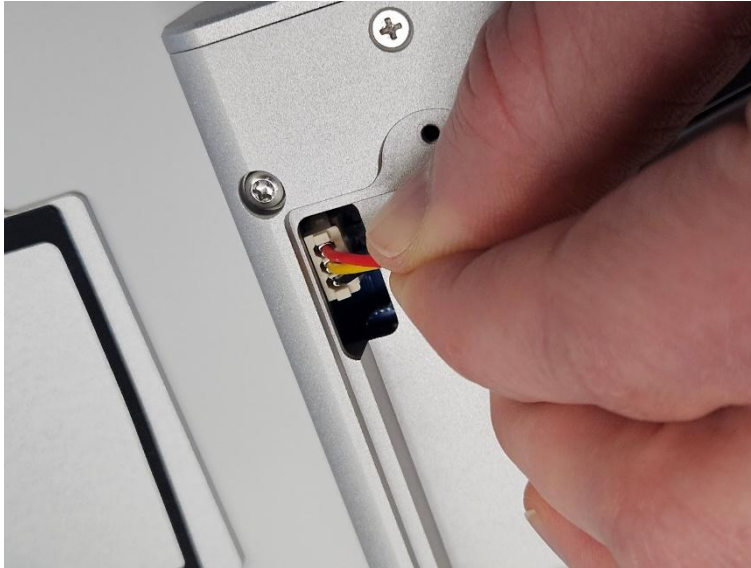
Figure 12 Unplugging the Li-Po battery
