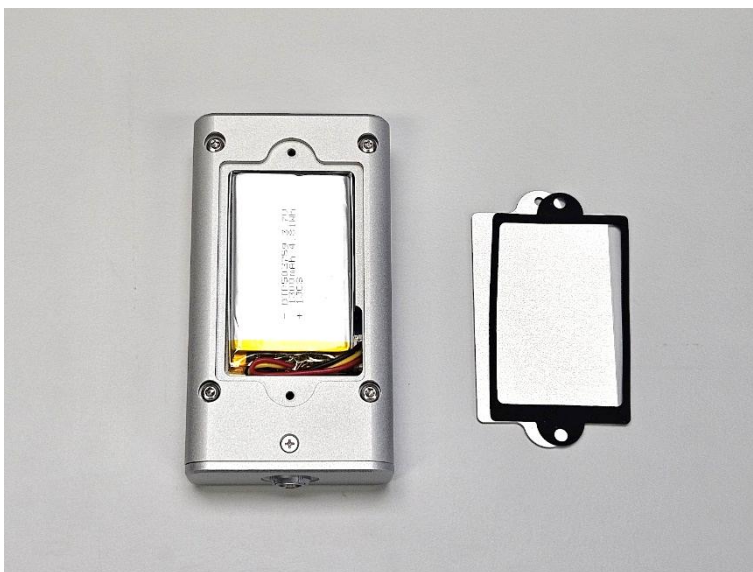
Figure 11 The battery lid removed.
