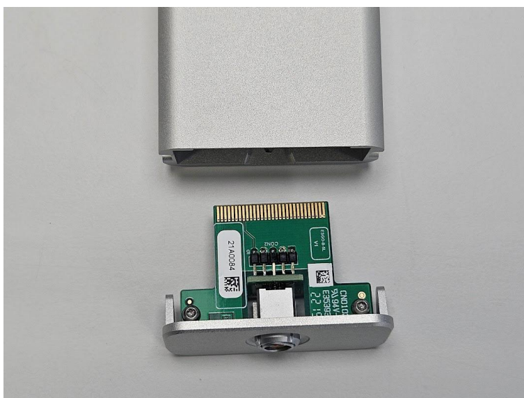
Figure 6 Replacing the Connection Module
