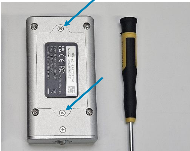
Figure 10 The two screws of the battery lid.
