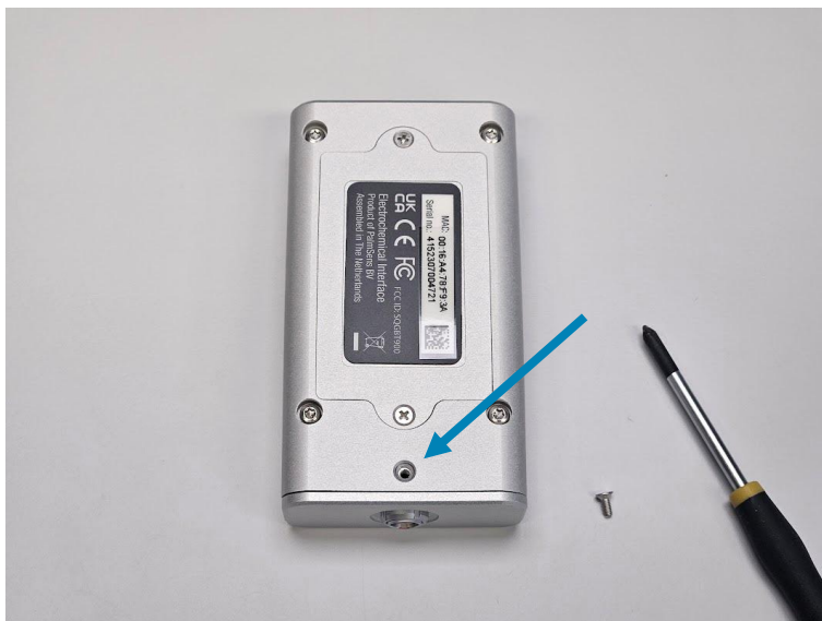
Figure 4 The Connection Module screw location.
