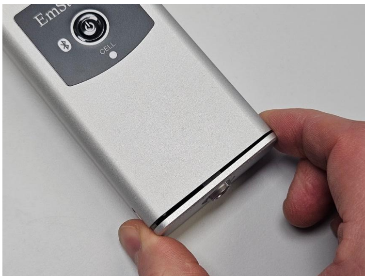
Figure 5 Pulling out the Connection Module.
