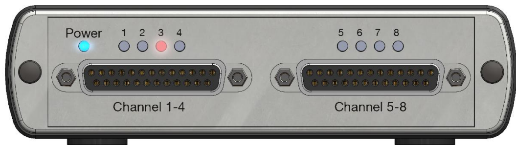
Figure 7 - Channel three being the active channel on the EmStat4 MUX
