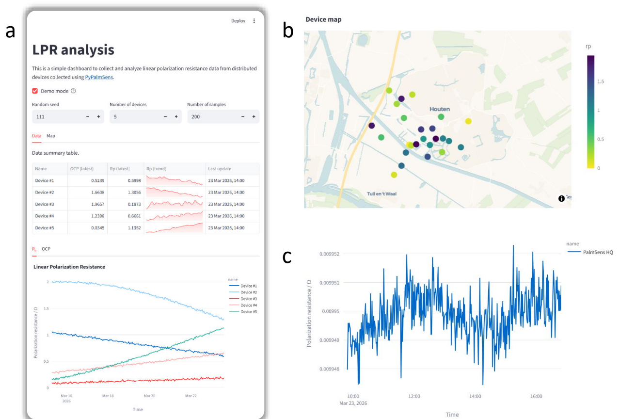
Figure 1. (a) Overview of the dashboard with semi-random generated mock data. The overview shows a table summarizing the data, and R_p or OCP charts. (b) Click on the 'Map' tab to show device locations and data on a map. Select points on the map to display the corresponding data in the R_p /OCP chart. (c) Example LPR data measured on an EmStat Pico using a dummy cell over the course of several days.
