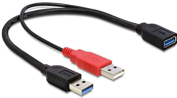
Figure 2 USB Y-Cable for extra power in case of using the BiPot module.
