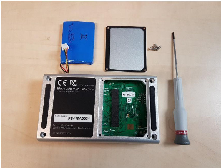
Figure 16 PalmSens4 with the battery lid removed.
