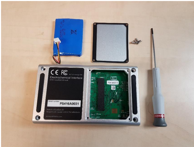
Figure 11 PalmSens4 with the battery lid removed.
