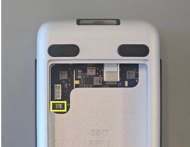
Figure 26 - EmStat4T bootloader emergency button
