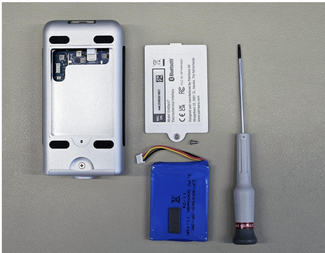
Figure 22 - EmStat4X with the battery lid removed.
