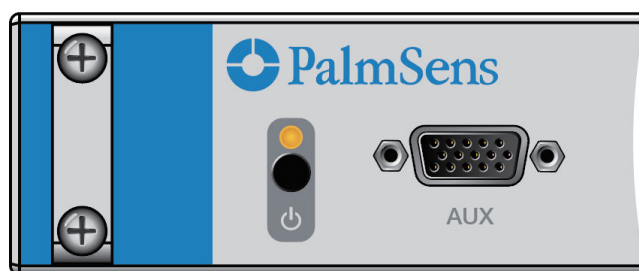
Figure 10. Power/Status LED on the front showing amber color when standby
