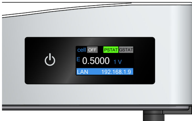
Figure 5. The assigned IP address showing in the blue bar on the display
