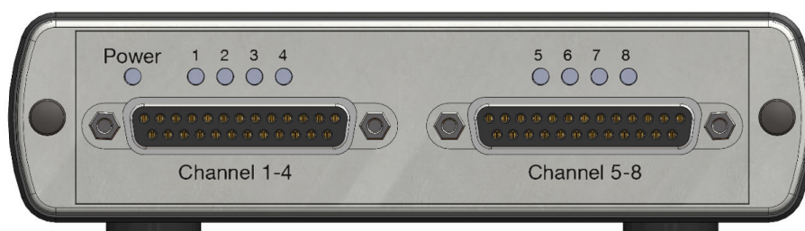
Figure 6. Two connectors for connecting eight electrochemical cells
