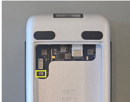
Figure 26. EmStat4T bootloader emergency button
