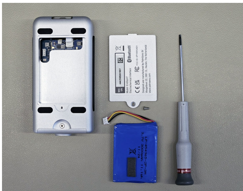
Figure 22. EmStat4X with the battery lid removed
