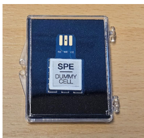
Figure 25. The SPE dummy cell supplied with the EmStat4T SPE version
