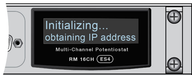
Figure 11. The display showing the internal Lablink is trying to obtain an IP address
