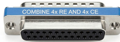
Figure 4. RE/CE Combiner for combining four counter and four reference electrodes
