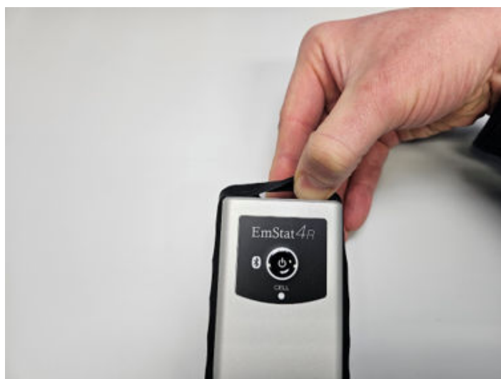
Figure 17. Pulling the rubber sleeve over the back of the housing
