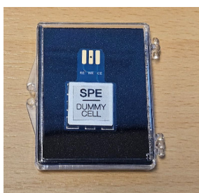
Figure 19. The SPE dummy cell supplied with the EmStat4R SPE version
