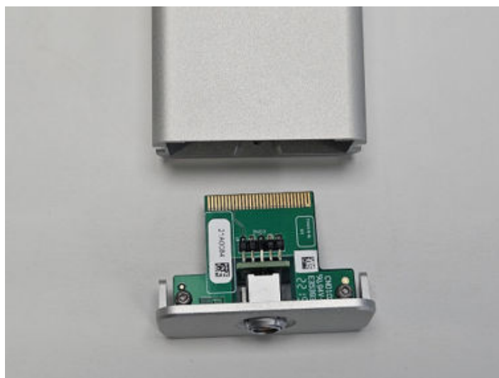
Figure 6. Replacing the Connection Module
